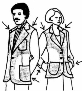
Interfacing used to support, reinforce & add shape to tailored garments
